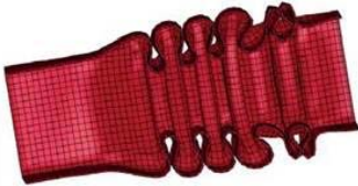
Figure 11: Buckling of a box girder under axial loading
