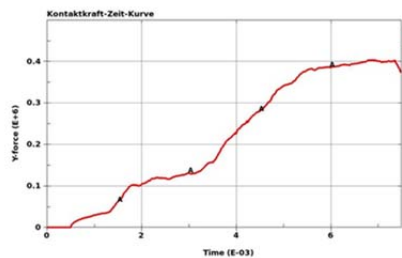
Figure 7: Analysis results of the optimized bumper
