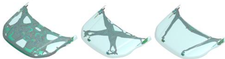
Figure 10 LS-TaSC Static Results
