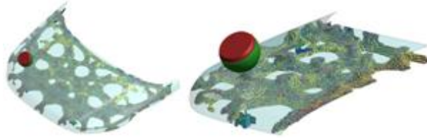
Figure 13 LS-TaSC Head Impact Result
