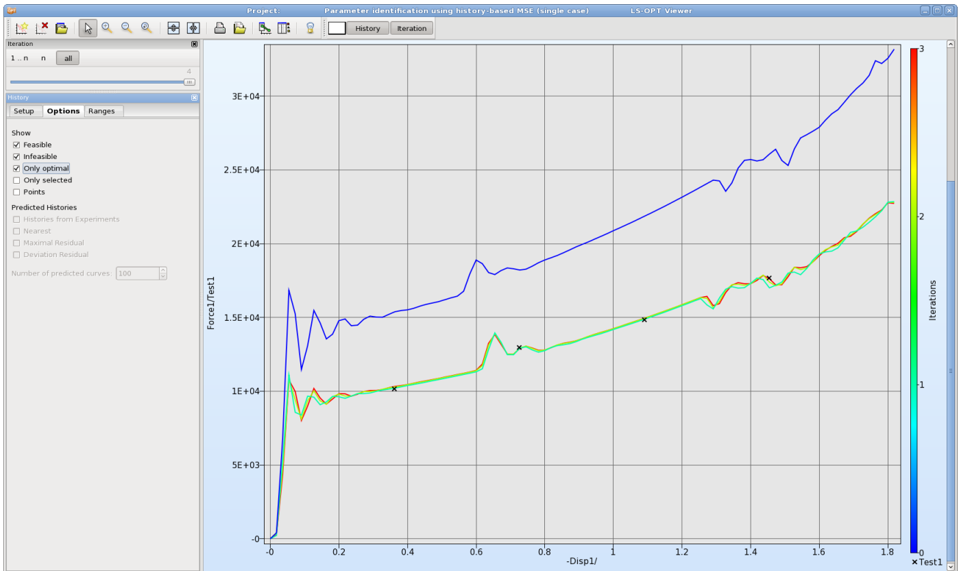
Figure 19-4: Target and computed curves, only optimal curves are displayed for all iterations
