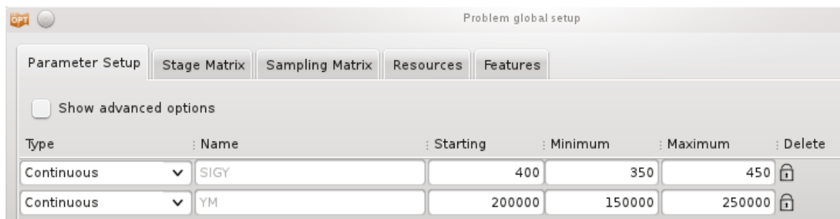
Figure 5-11: Outer level global setup. SIGY and YM are automatically detected in the input file (i.e. inner level .lsopt file) and locked as they are Transfer Variables in the inner level.
