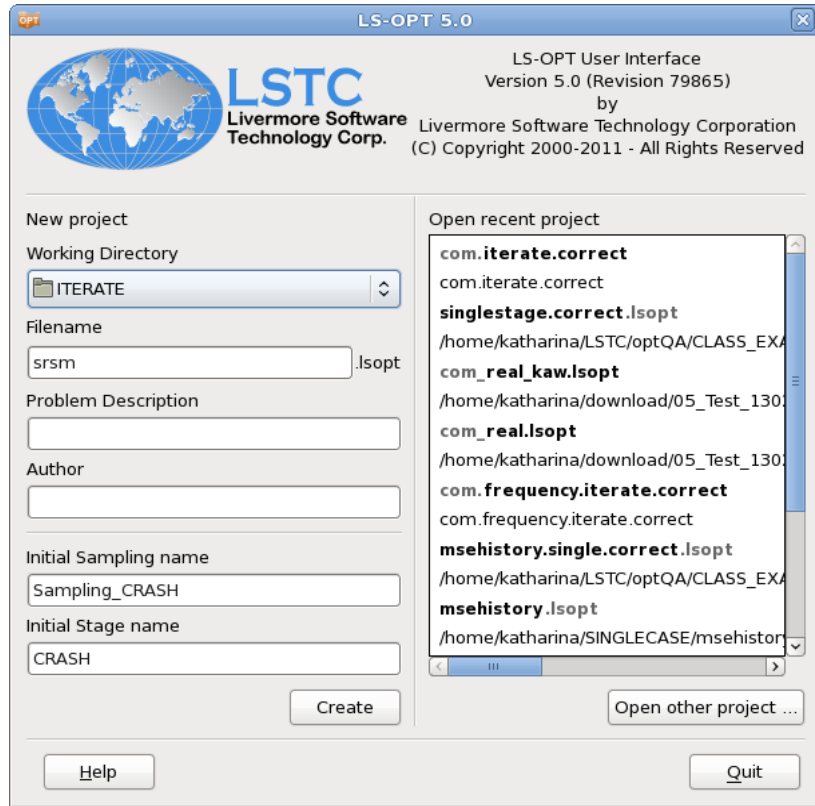
Figure 2-1: LS-OPT Startup dialog. Select the working directory, enter a name for the LS-OPT project file and a name for the initial sampling and initial stage to generate a new project.
