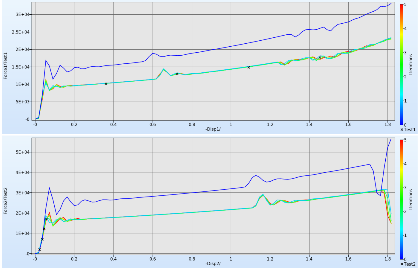
Figure 17-12: Comparison of optimal force-displacement curves and test data. The simulation curves are colored by iteration
