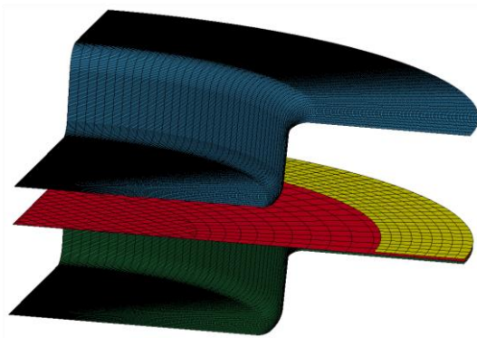
Figure 16-65: Quarter segment of FE model: tools and blank
