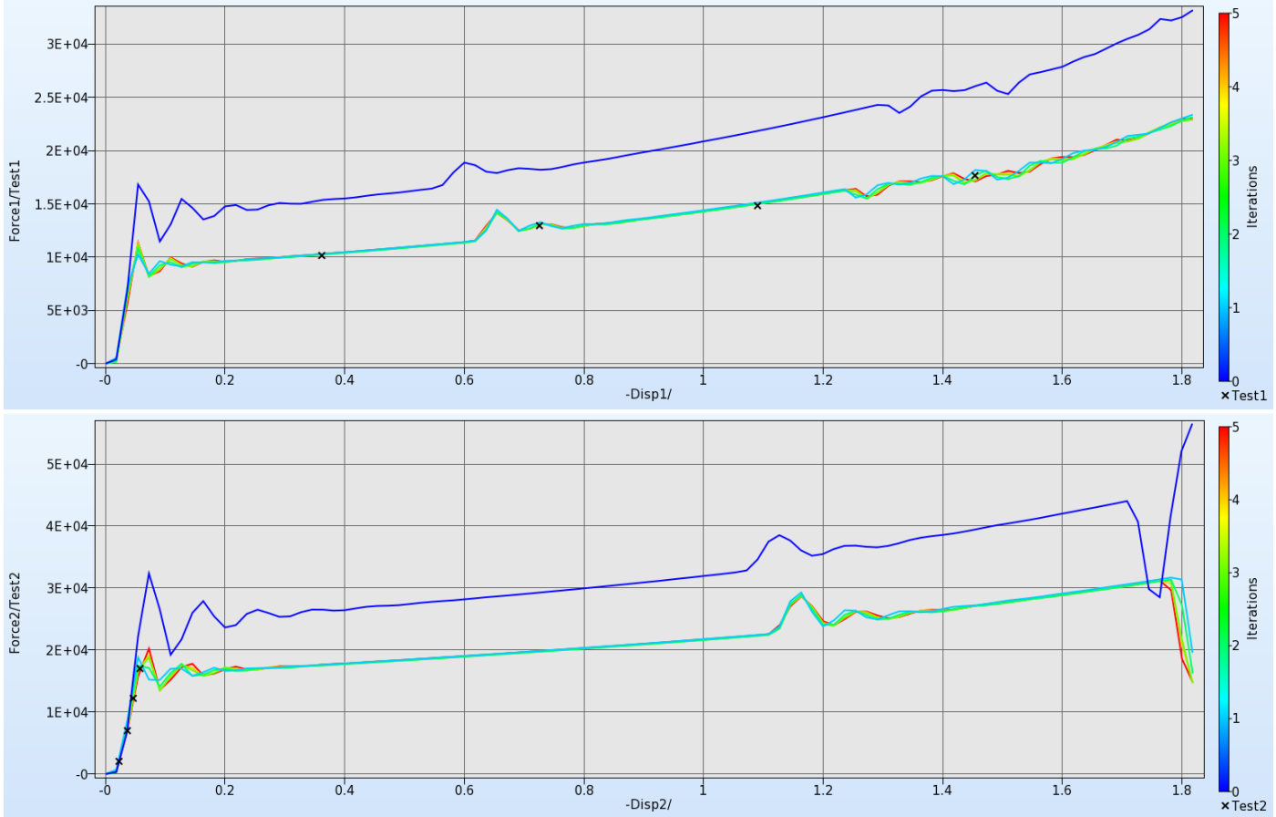
Figure 18-12: Comparison of optimal force-displacement curves and test data. The simulation curves are colored by iteration
